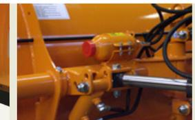
**HAG - Hydraulic pistons for angle adjustment**
