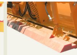
**HPS - Hydraulic device for polyurethane scraping edge**
